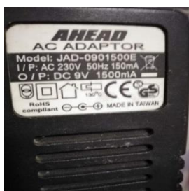
Fig.(10) The power supply used for TECs
