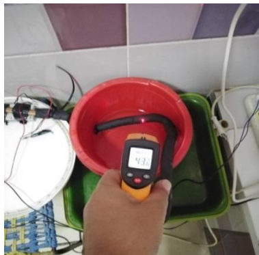
Fig. (14) Water temperature after passing the system
