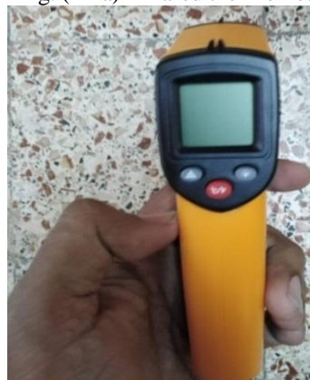
Fig. (12-b) Infrared thermometer control panel and its monitor
