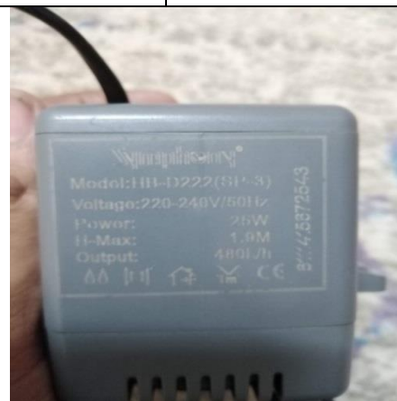
Fig. (8-a) the submerged pump used for the test
