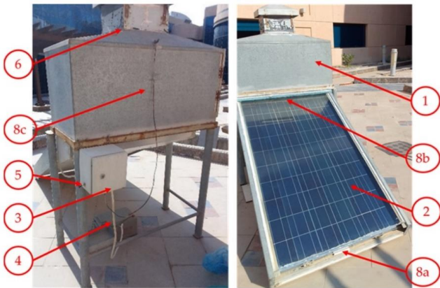
Figure 10. Main parts of the SD, 1. drying chamber, 2. PV/T SC, 3. solar charger, 4. battery, 5. controller, 6. Suction fan, 8. DHT22 sensors [30].
