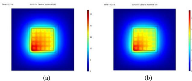
Fig. 8. Behavior of ESP in the case of soil with single type of structure; (a) pure clay at depth 0.5 m, (b) pure clay at depth 0.75 m
