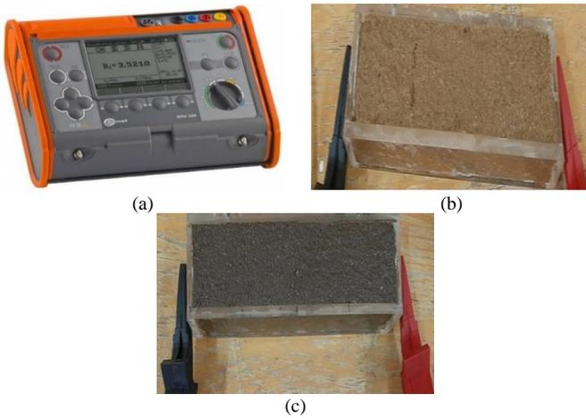
Fig. 1. Soil electrical resistance measurement: (a) Sonel (MRU-200) soil resistance measurement instrument. (b) soil box model with sandy sample (c) soil box model with clay sample
