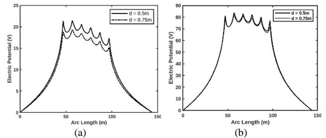
Fig. 7. ESP in the case of soil with single type of structure; (a) the central profile of pure clay at depth 0.5 & 0.75m, (b) the central profile of pure sand at depth 0.5 & 0.75m
