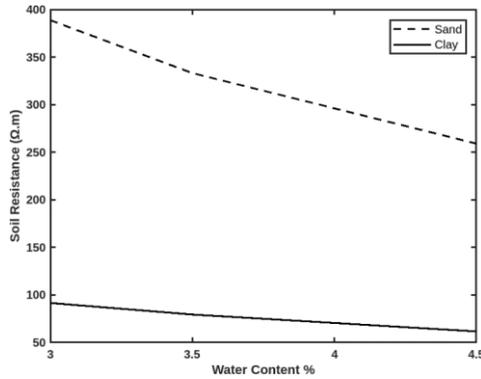
Fig. 6. Relation between the water content and the resistance of sandy and clay soils
