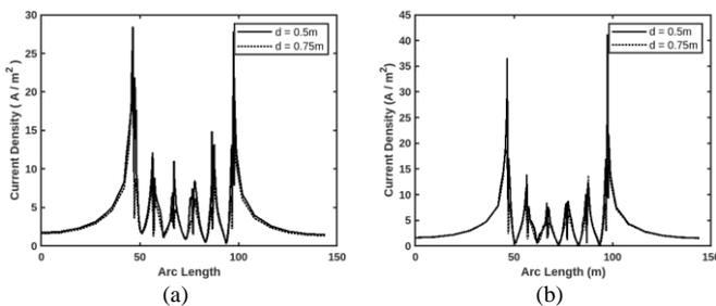
Fig. 9. ground current density in the case of soil with single type of structure; (a) Central profile of pure clay at depth 0.5 & 0.75m, (b) Central profile of pure sand at depth 0.5 & 0.75m
