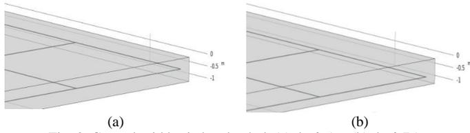
Fig. 3. Ground grid buried at depth d; (a) d =0.5m, (b) d =0.75m
