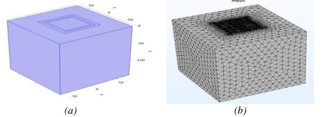
Fig. 2. (a) Simulator model consists of ground grid and the soil (b) Mesh elements of FEM
