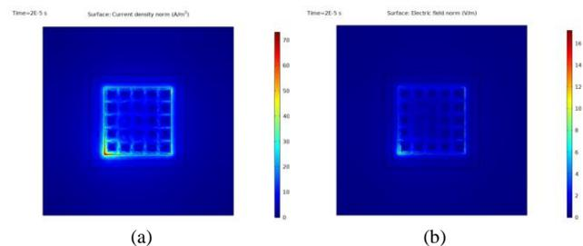
Fig. 10. Behavior of the electric field in the ground grid in the case of soil with single type of structure; (a) Clay at depth 0.5 m, (b) Clay at depth 0.75 m
