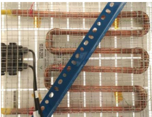
FIGURE 2. WATER COOLING COPPER PIPE [15].
