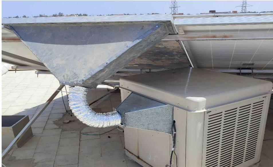
Fig. 2. humidified air-cooling design
